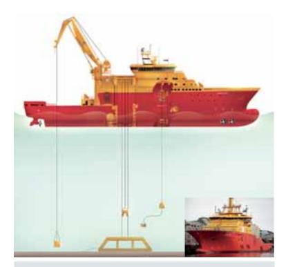
**Research and development** The challenging nature of offshore operations means that load handling must often be undertaken by a wide variety of specialised systems, not just cranes. Many subsea lifts require advanced module handling systems which can offer very precise handling of critical loads – something which is vital when mating subsea units on the seabed or in the vicinity of other delicate equipment. This precision becomes even more challenging in rough seas.
